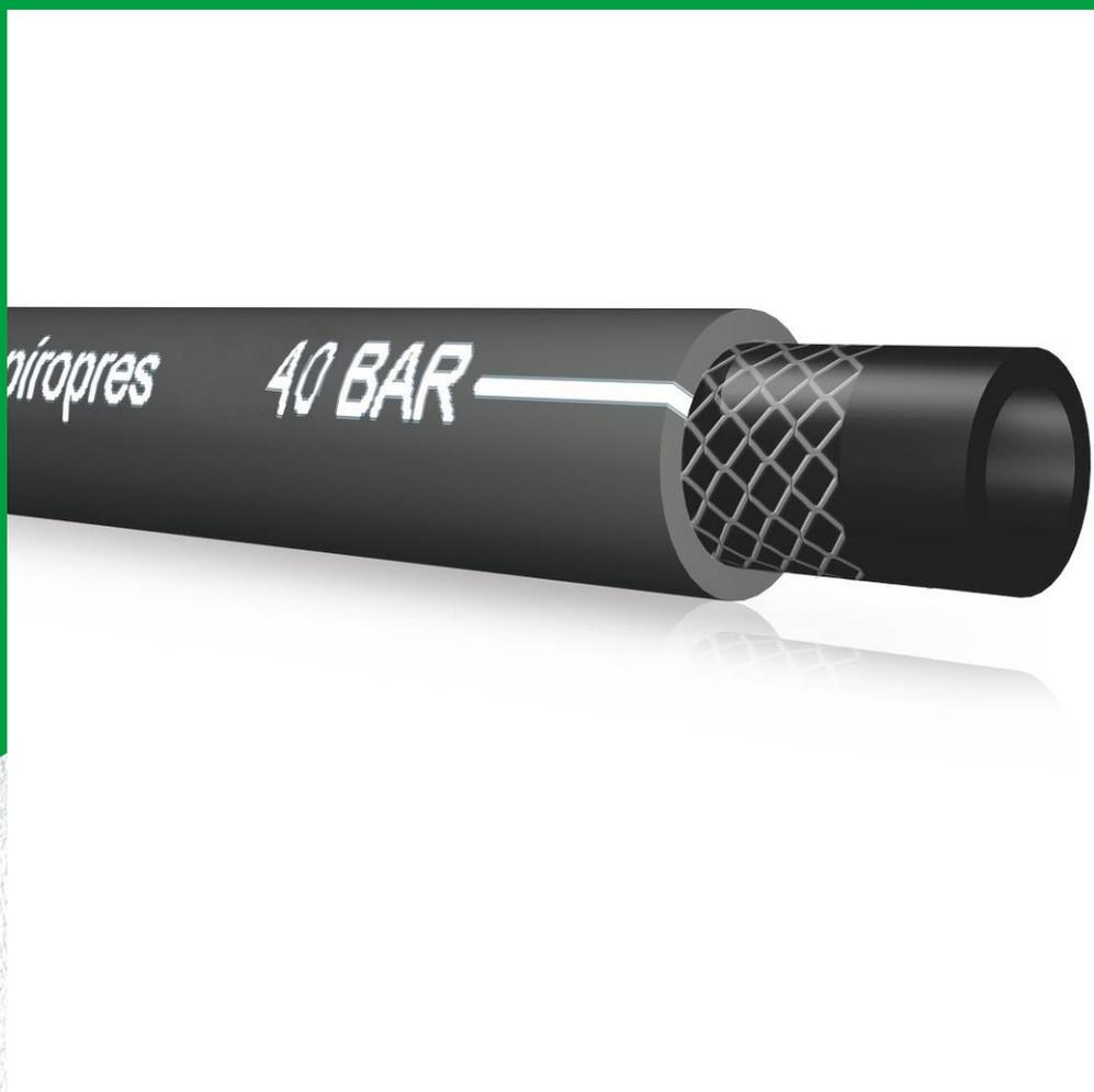
Tube fabricated by co-extrusion of primary quality vinyl products, with polyester fabric reinforcement. Good resistance to atmospheric agents and to the passage of chemical products according to the standard properties of PVC.
